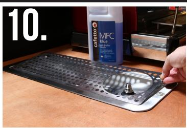
Reassemble the Drain Tray,
